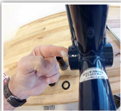
1. Thoroughly clean the bottom bracket shell. Apply a thin layer of grease to inner shell.
