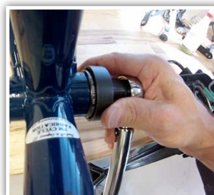
6. Use Park Tool BBT-69 to thread non-drive side cup into frame until flush. Using torque wrench, fully tighten to 35-50Nm.
