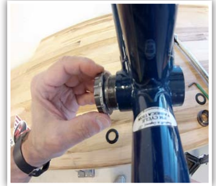
3. Insert drive side cup and center sleeve into frame.
