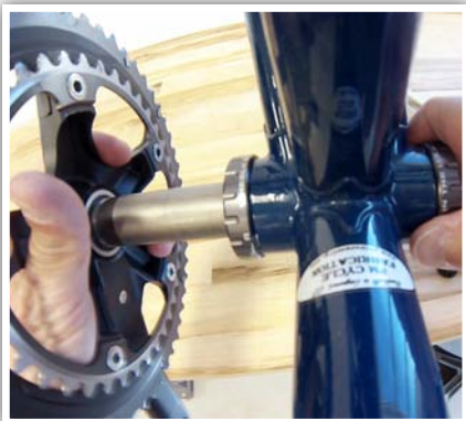
7. Install right crank arm, making sure outer dust seal is installed.
