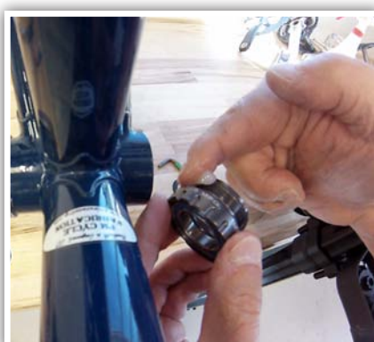
5. Apply a thin layer of grease to cup.
