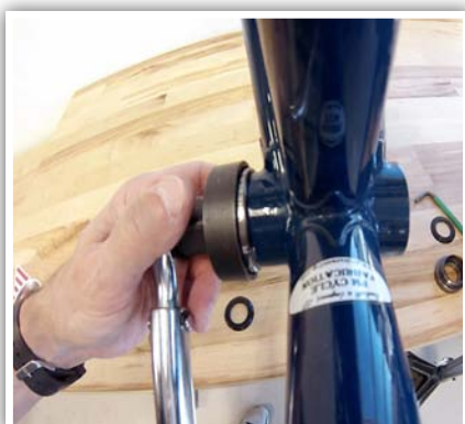
4. Use Park Tool BBT-69 to thread drive side cup into frame until flush. Using torque wrench, fully tighten to 35-50Nm.
