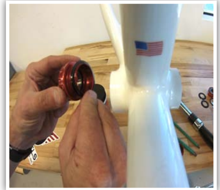
3. Insert drive side cup and center sleeve into frame, add supplied spacers as necessary to achieve proper bottom bracket width.
