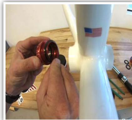
3. Insert drive side cup and center sleeve into frame, add supplied spacers as necessary to achieve proper bottom bracket width.
