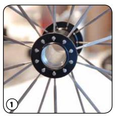
REMOVE OLD/ WORN BEARINGS FROM HUB/ BOTTOM BRACKET WITH WHEELS MFG. BEARING REMOVAL TOOL (BRT-I) OR APPROPRIATE REMOVAL DEVICE.
