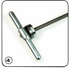
PLACE BEARING ONTO BEARING ADAPTOR, ENSURING IT IS SEATED CORRECTLY. INSERT HANDLE WITH BEARING AND ADAPTOR INTO HUB. PLACE OPEN BORE ADAPTOR ONTO THEADED HANDLE FROM OPPOSITE SIDE, SECURING WITH OTHER HANDLE.
