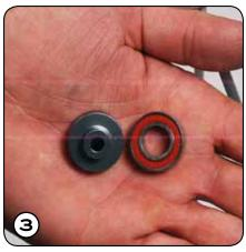
PURCHASE APPROPRIATE SIZE BEARING ADAPTOR FOR THE BEARING YOU WISH TO REPLACE. FOR LONGEST BEARING LIFE, INSTALL ONE BEARING AT A TIME. INSTALL OPEN BORE BEARING ADAPTOR ONTO THREADED HANDLE.
