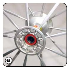
REMOVE HANDLE AND ADAPTOR FROM HUB. FIRST BEARING IS INSTALLED. REPEAT THIS PROCESS FOR THE SECOND BEARING.
