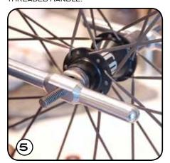
TIGHTEN HANDLE UNTIL BEARING BOTTOMS OUT AGAINST BEARING STOP. DO NOT OVER TIGHTEN.
