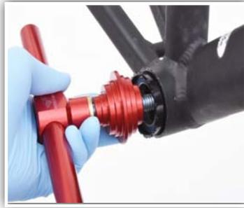
5. Insert one BB adapter into drive side bearing. Match the correct size step on the drift with bearing inner diameter. Slide press handle + rod thru BB adapter and cup.
