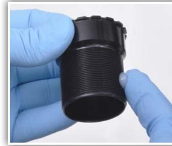
2. Apply a thin layer of high quality grease to all threads on both cups.
