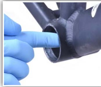
1. Thoroughly clean frame's bottom bracket shell. Do not install cups dry. Apply a thin layer of high quality, carbon-safe grease or anti-seize compound to inside surface of the shell.
