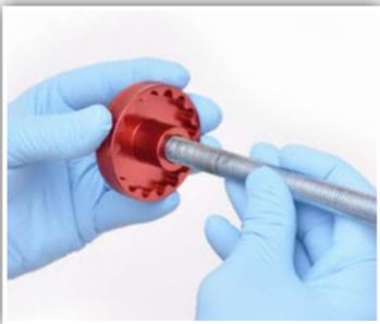
9. For internal bearing BB cups with narrow 48.5mm 16-notch flanges, using the narrow socket with the press handles, rod and drifts will allow you to securely hold the socket tools on the BB cups. Thread the narrow socket tool onto the threaded rod.
