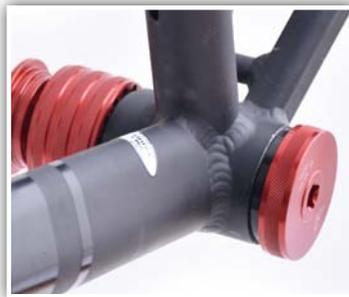
10. Insert narrow socket + rod through non-drive side cup. Slide the larger BB socket over the rod and up against the drive side cup. Engage the splines on both sockets with each cup.
