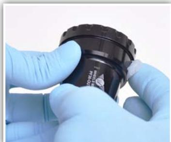
3. Apply a thin layer of high quality, carbon-safe grease or anti-seize compound to outside surface of each BB cup.
