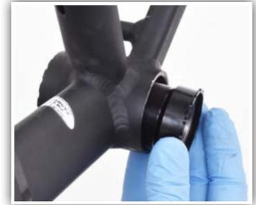
8. Insert non-drive side cup by hand and turn clockwise until threads begin to engage. Do not cross-thread cups. Check that any internal wires or hoses are out of the way of the cup.
