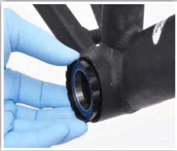
4. Insert drive side cup (female threads) into frame by hand. If cup fully inserts by hand, this is OK and move on to step 8. Check that any internal wires or hoses are out of the way of the cup.
