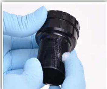
2. Apply a thin layer of high quality grease to all threads on both cups.
