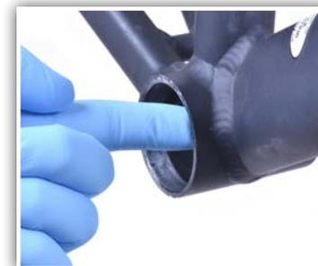
1. Thoroughly clean frame's bottom bracket shell. Do not install cups dry. Apply a thin layer of high quality, carbon-safe grease or anti-seize compound to inside surface of the shell.
