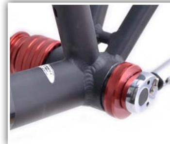
12. Attach torque wrench to the narrow socket and tighten cups to 35 - 50Nm.
