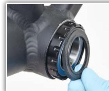
11. Bottom bracket is now installed. Install crankset per crank manufacturer's instructions. Outer silicone dust seals are placed directly against bearings. For added sealing, apply grease between seal and bearing.
