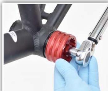
9. Continue to turn cup clockwise until flush against the outer face of frame. Finish tightening cups using Wheels Mfg BB Socket [BOTOOL-48-44] to 35Nm - 50Nm.
