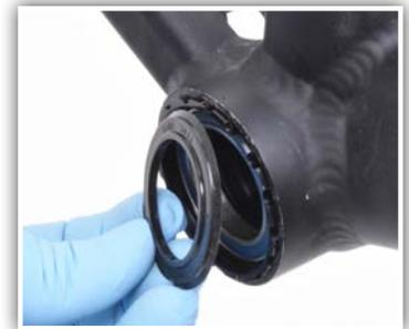
13. Bottom bracket is now installed. Install crankset per crank manufacturer's instructions. Outer silicone dust seals are placed directly against bearings. For added sealing, apply grease between seal and bearing.
