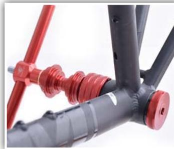
11. Add the BB drifts to take up any additional space, then spin on a handle until the stack is snug enough to hold the sockets in place. **Do not overtighten!**
