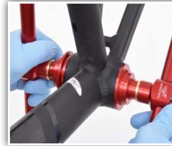
7. Spin on second press handle and fully tighten until drive side cup is flush with frame.
