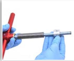
2. Slide the bearing extractor pusher onto a Wheels Mfg Universal BB Press [PRESS-7 or PRESS-7-PRO] rod. Next, add the matching adapter with the tapered end of the adapter opposite the pusher.
