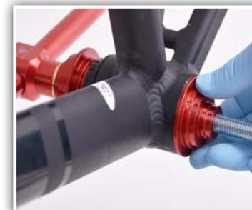
6. Slide second BB adapter onto threaded rod and into the opposite side of the bottom bracket shell. Match the correct step size with the BB shell inside diameter. Adapter should fit with little to no play.
