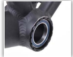
12. Remove press handles and adapters from cups. Bearing is now installed.
