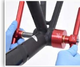
5. Spin on second handle and tighten handles together until you feel the bearing pop out of the cup.
