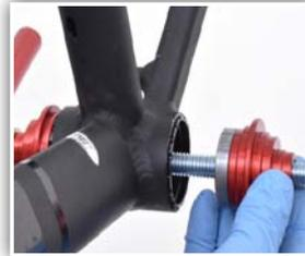
10. Slide new bearing onto second BB adapter, matching up the correct size step on the adapter with the bearing ID. Slide both onto press rod.
