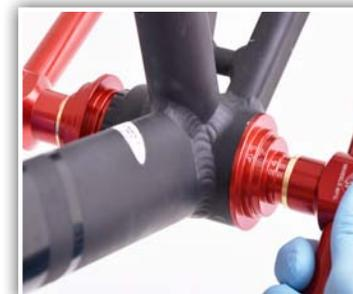
7. Spin on second press handle and fully tighten until drive side cup is flush with frame.
