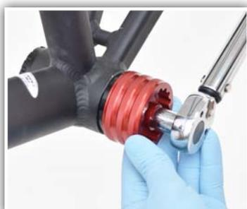
9. Continue to turn cup clockwise until flush against the outer face of frame. Finish tightening cups using Wheels Mfg BB Socket [BBTOOL-48-44] or Flat Wrench [WRENCH-BB48-44]. Tighten cups 35Nm - 50Nm.
