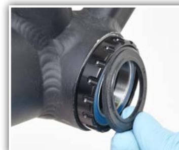
12. Outer silicone dust seals are placed directly against bearings. For added sealing, apply grease between seal and bearing.
