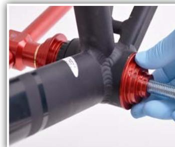
6. Slide second BB adapter onto threaded rod and into the opposite side of the bottom bracket shell. Match the correct step size with the BB shell inside diameter. Adapter should fit with little to no play.
