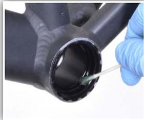
8. Clean and dry bearing bore in cup. Apply thin film of Loctite 603 retaining compound to cup.
