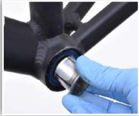
1. Insert appropriate size extractor into bearing. Push extractor completely in until you feel it snap in place.
