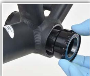
8. Insert non-drive side cup by hand and turn clockwise until threads begin to engage. Do not cross-thread cups. Check that any internal wires or hoses are out of the way of the cup.
