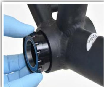
4. Insert drive side cup (female threads) into frame by hand. If cup fully inserts by hand, this is OK and move on to step 8. Check that any internal wires or hoses are out of the way of the cup.
