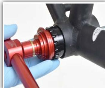
5. Using Wheels Mfg Universal Bottom Bracket Press [PRESS-7 or PRESS-7-PRO], insert one BB adapter into drive side bearing. Match the correct size step on the drift with bearing inner diameter. Slide press handle + rod thru BB adapter and cup.
