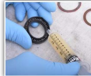
3. Pack bearing with new, clean bearing grease [GR-001].
