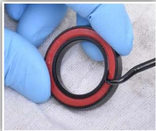
1. Lift up seal using a utility knife or pick. If servicing bearings outside of BB cups, remove both seals. Clean seals and set aside. For Angular Contact bearings, note which side takes the black seal.
