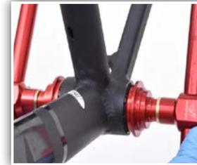
11. Spin on second handle and tighten handles together until the bearing is seated in the cup.
