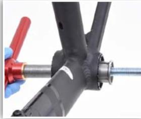
3. Insert handle, rod, pusher and adapter into the backside of the bearing you are removing.
