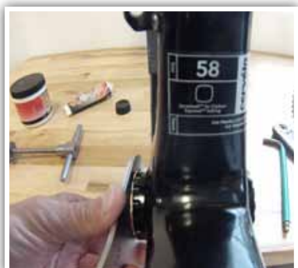
7. Using 16 notch wrench ( WRENCH-BB48-39 ), fully tighten cup. Approximate torque 35-50Nm.
