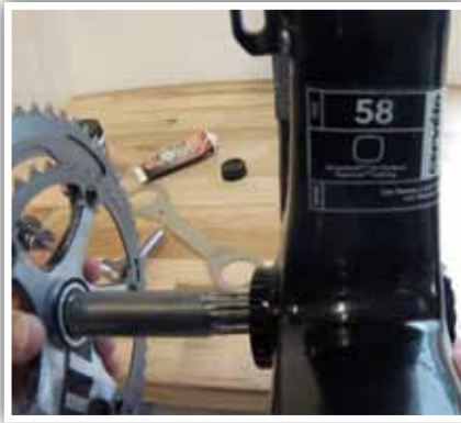
8. Install right crank arm, making sure wave washer and outer dust seal is installed. Wave washer goes between the crank and the outer dust seal.
