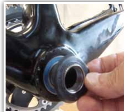
9. Make sure outer dust seal is in place before installing left crank arm.
