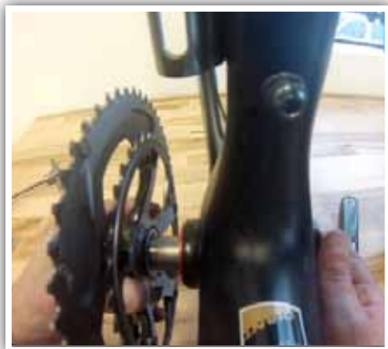
7. Install right crank arm, making sure wave washer and outer dust seal is installed.
