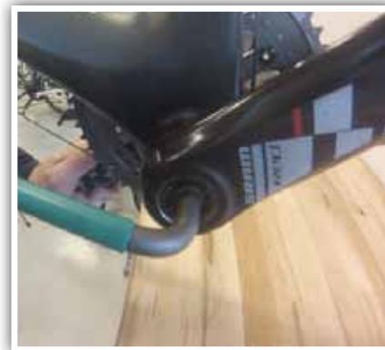
9. Install left crank arm, tighten crank to manufacturer specifications.
