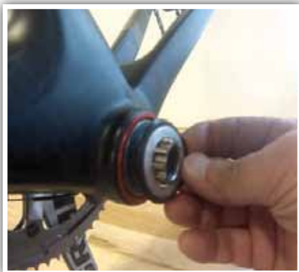
8. Make sure outer dust seal is in place before installing left crank arm.
