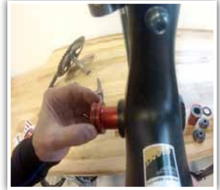
3. Insert drive side cup into frame.
