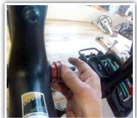
6. Use PRESS-1 or PRESS-4 with one 2437 bearing drift (non-drive side) and one GXP-LEFT drift (non-drive side) to press cup into frame. Fully tighten until cup is flush with the frame.
