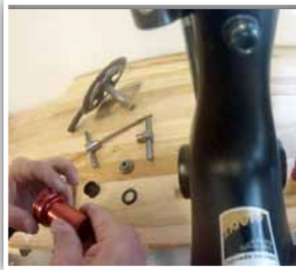
2. Apply a thin layer of high quality grease, PTFE or anti-seize compound to BB cup surface.
