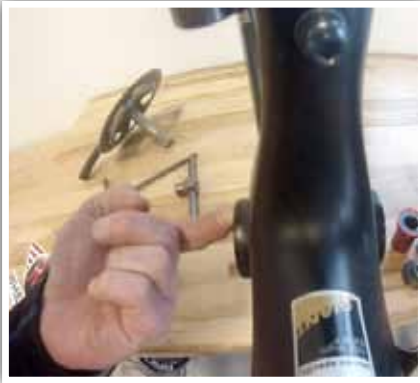
1. Thoroughly clean the bottom bracket shell. Do Not install cups dry. Apply a thin layer of high quality grease, PTFE or anti-seize compound to inside surface of the shell.
