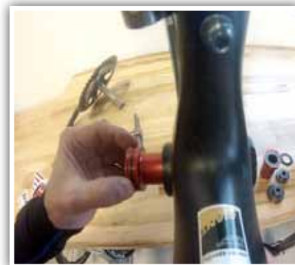
3. Insert drive side cup into frame.
