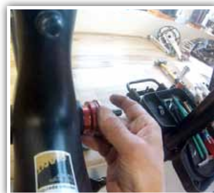
6. Insert non-drive side cup into frame by hand until threads begin to engage. Pay careful attention to not cross-thread cups.
