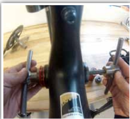
4. Use PRESS-1 or PRESS-4 with one 2437 bearing drift (drive side) and one PF30-OB-24 drift (non-drive side) to press cup into frame. Fully tighten until cup is flush with the frame.
