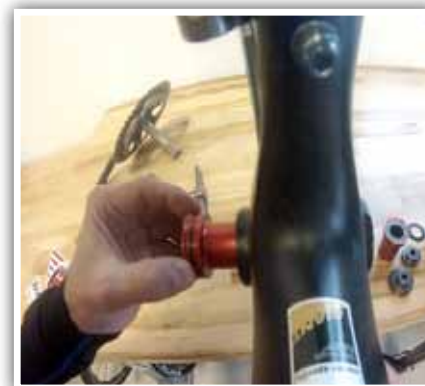
3. Insert drive side cup into frame.
