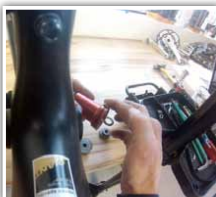
5. Apply a thin layer of grease, PTFE or anti-seize compound to non-drive side cup outer surface.
