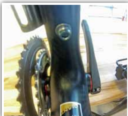
10. Add spacers as necessary to take up any play, remove spacers as necessary if binding occurs.
