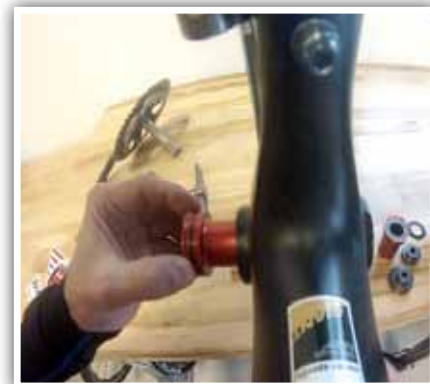
3. Insert drive side cup into frame.
