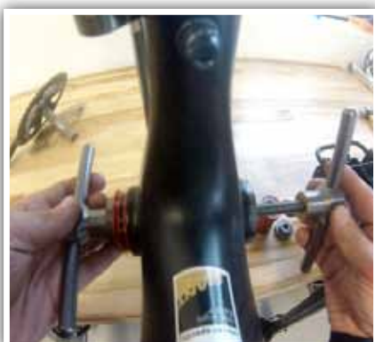
4. Use PRESS-1 or PRESS-4 with one 2437 bearing drift (drive side) and one BB86-0B drift (non-drive side) to press cup into frame. Fully tighten until cup is flush with the frame.
