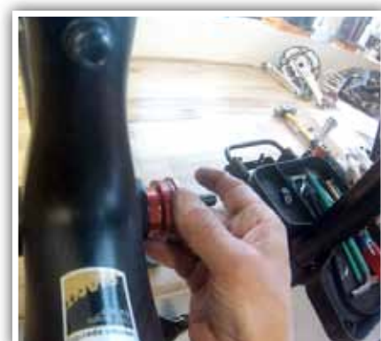
6. Use PRESS-1 or PRESS-4 with two 2437 bearing drifts to press cup into frame. Fully tighten until cup is flush with the frame.
