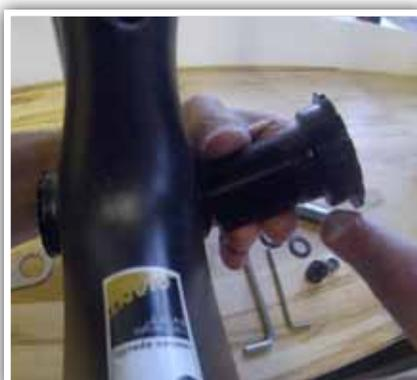
5. Apply grease to threads. **Do not use thread locking compound, PTFE or anti-seize on the threads.**
