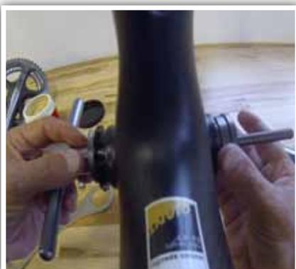
4. Use PRESS-1 or PRESS-4 with one 2437 bearing drift (drive side) and one BB86-OB-24 drift (non-drive side) to press cup into frame. Fully tighten until cup is flush with the frame.
