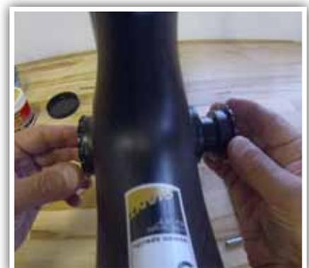
6. Insert non-drive side cup into frame by hand until threads begin to engage. Pay careful attention to not cross-thread cups.
