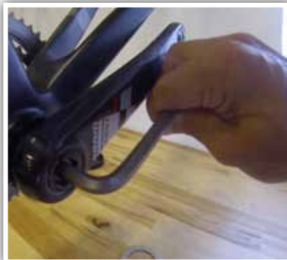
10. Install left crank arm, tighten crank to manufacturer specifications.
