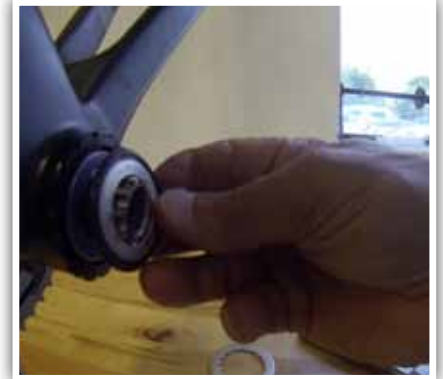
9. Make sure outer dust seal is in place before installing left crank arm.
