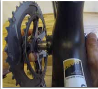
8. Install right crank arm, making sure wave washer and outer dust seal is installed.
