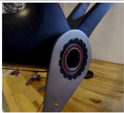
7. Using 16 notch wrench (48.5mm), fully tighten cup. Approximate torque 35-50Nm.
