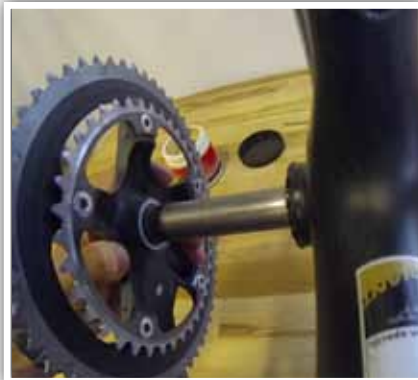
8. Install right crank arm, making sure outer dust seal is installed.
