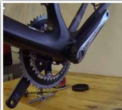
11. Add spacers as necessary to take up any play, remove spacers as necessary if binding occurs.
