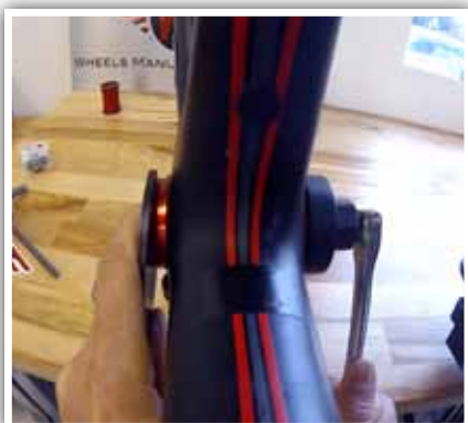
7. Using torque wrench, tighten cups to 35-50 Nm.
