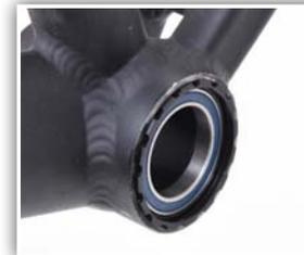
12. Remove press handles and adapters from cups. Bearing is now installed.
