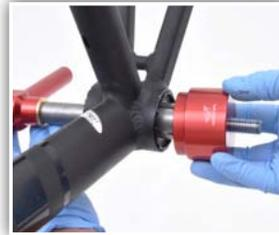
4. Select a sleeve size that has a larger ID than the bearing's OD. Slide receiver cup + reducer sleeve over the rod and up against cup.
