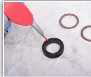
2. Flush out old grease with a de-greaser. Dry bearing to remove any traces of degreaser.
