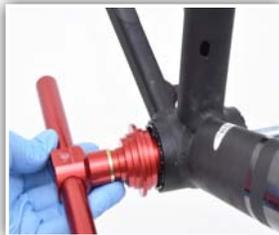
9. Slide one BB adapter over the press rod. Match the correct size step on the adapter with the cup or bearing. Insert into bearing or cup opposite the bearing you are installing.
