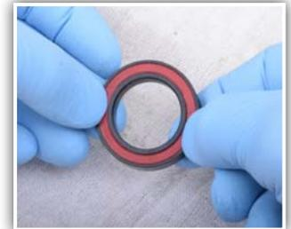
4. Lightly press seals onto bearing. Seals should sit flush to the outer face of the bearing races.
