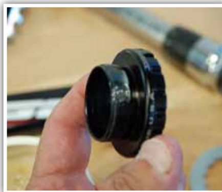
5. Apply a thin layer of grease to cup.
