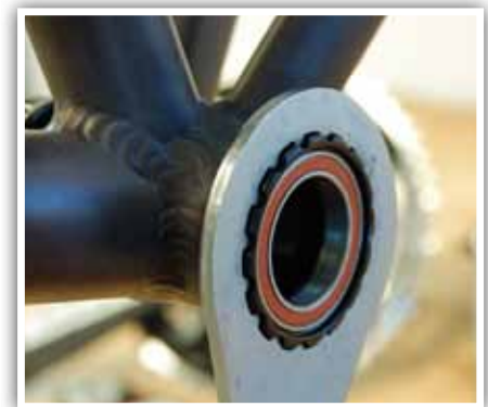
6. Use 16-notch BB tool - 48.5mm OD to thread non-drive side cup into frame until flush. Using torque wrench, fully tighten to 35-50Nm.
