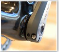
Take up any play in your cranks with supplied Crank Spindle Spacers. Place the spacers as needed.
