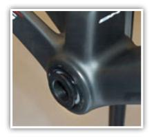
1. If not already installed, press the PF30 bottom bracket cups into frame. Remove outer dust covers, if present. (Do not remove the bearing seals).
