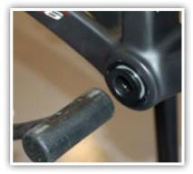
2. Start inserting adapters into bottom bracket bearings by hand. Seat adapters using a rubber mallet.
