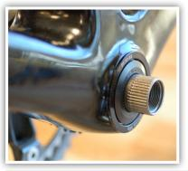
Install crank spindle through the adapters and tighten per manufacturer's instructions.
